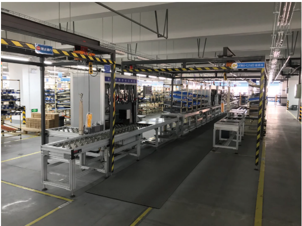
ACB生产线 ACB assembly line
