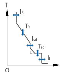
**多曲线过载长延时保护动作延时时间表****Action delay schedule of multi curve overload long delay protection**
