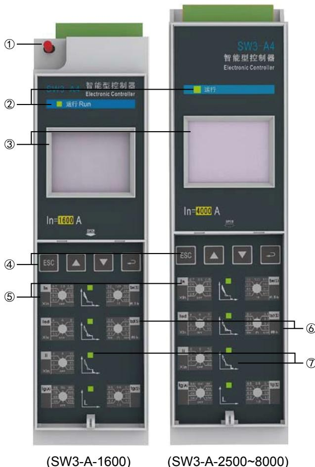
SW3-A3, SW3-A4 intelligent controller to protect the main circuit power supply; A3 type to provide selective long delay, short delay, instantaneous three sections of protection; A4 type on the basis of A3 to increase the selective ground fault protection; Display interface to increase the LCD screen; Applicable to the chassis current 1600A ~ 8000A circuit breaker.
