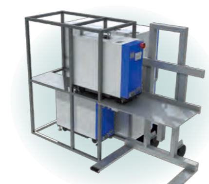
• Pump lifter for exchange Dedicated lifter for safe pump exchange
