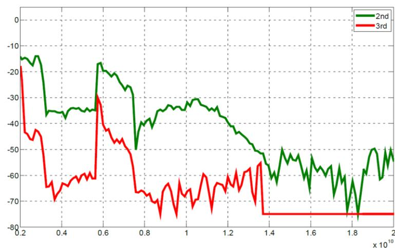
Harmonic output power [dBc] vs. frequency [Hz]
