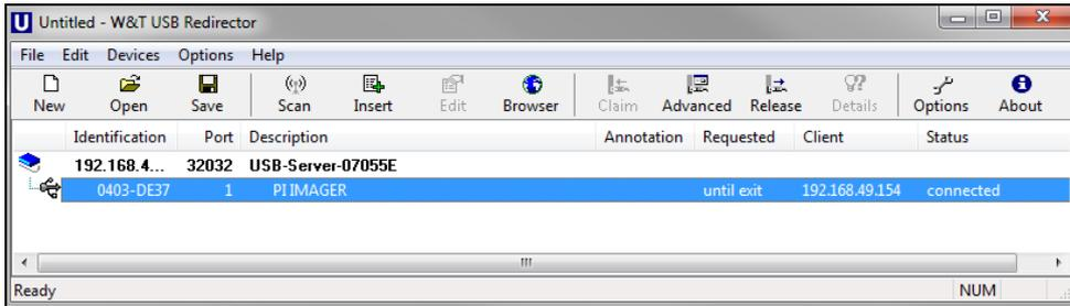
The device (IR camera PI, CTvideo or CSvideo) can now be used in the same way as it would be connected directly to a local USB port of your PC. The program **Redirector** can be minimized – if you close the window, the **Redirector** will be automatically terminated.
