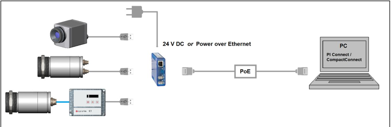
On a direct connection to a PC both, the USB server as well as the PC must use a fixed IP address. There is no DHCP server available. Accomplish the following settings on your PC once (depending on the operating system the procedure can differ from the here shown – the following description refers to a Windows 7 system).
