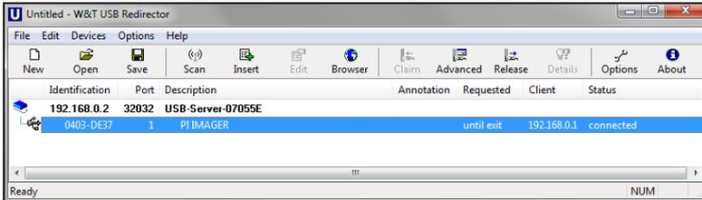
The device (IR camera PI, CTvideo or CSvideo) can now be used in the same way as it would be connected directly to a local USB port of your PC. The program **Redirector** can be minimized – the connection will be determined if you close the window.
