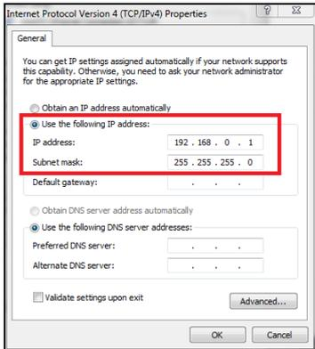
If you want to switch between a user-defined IP address and a DHCP server, the following alternative configuration is recommended: Under the **General** tab choose **Obtain an IP address automatically**, and on the **Alternate Configuration** tab, click **User configured** and enter a user defined IP address:
