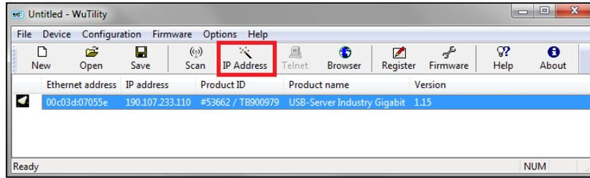
8. The standard setting of the USB server is DHCP. On a direct connection to a PC set a static IP address to the device. Take care that the network part of the address is identical to the network part of the IP address of the connected PC (therefore: **192.168.0**). The host part must have a different digit than the user-defined IP address of your PC (for example: 192.168.0.2):
