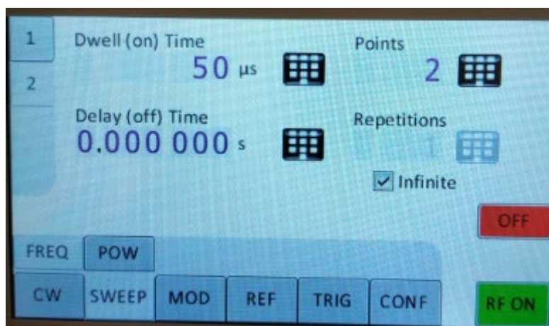
Figure 7-t Displays shown for the frequency sweep configuration
