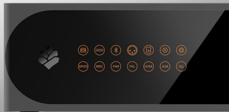
④ SGD1 is successfully connected to the network, and the upgrade is started. The icon is all bright when upgrading
