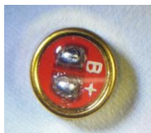
BY4015BOB-CR K \Phi 4.0 \times 1.5 ( mm ) Sensitivity:-42 \pm 3dB B SNR: 60dB
