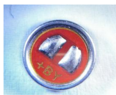
BY6027FOB-CR K \Phi 6.0 \times 2.7 ( mm ) Sensitivity:-42 \pm 3dB B SNR: 60dB
