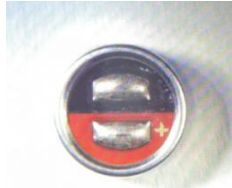
BY6027FOB-CR \Phi 6.0 \times 2.7 ( mm ) Sensitivity:-42 \pm 3dB B SNR: 60dB A
