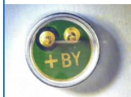
BY6050FOP2.8-CRK \Phi 6.0 \times 5.0 ( mm ) Sensitivity:-42 \pm 3dB B SNR: 60dB A
