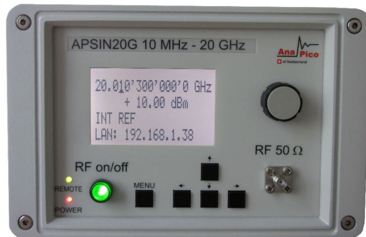
Figure Error! No text of specified style in document.-q APSIN Front Panel
